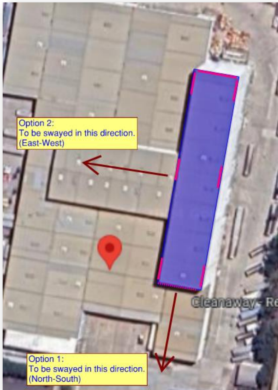
Figure 4: Option 1 & Option 2 for demolition
